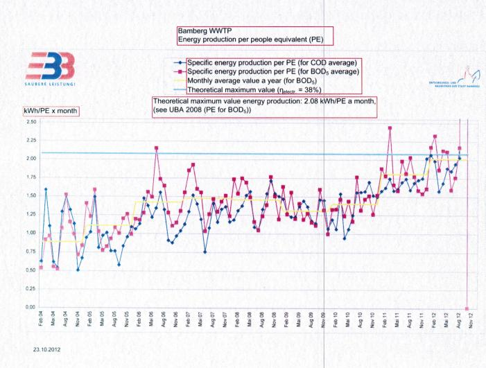
Figure: Energy production per people equivalent (PE) on Bamberg WWTP
