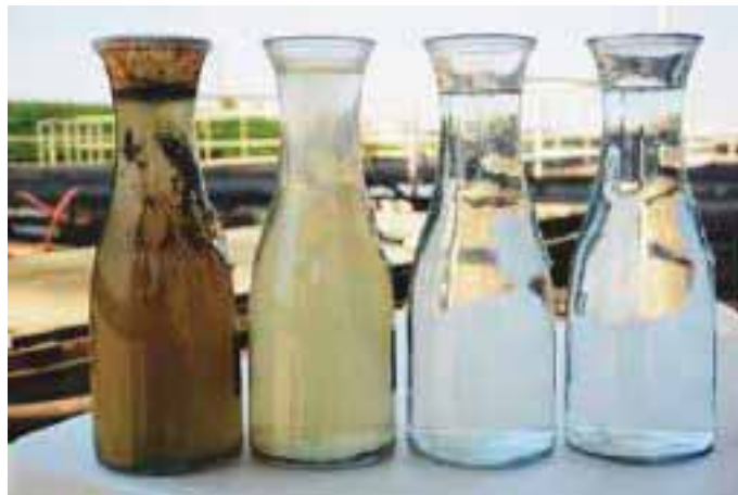
Produced water at varying stages of treatment using the ECOPOD system, which incorporates OriginClear's EWS technology. Photo by OriginClear
