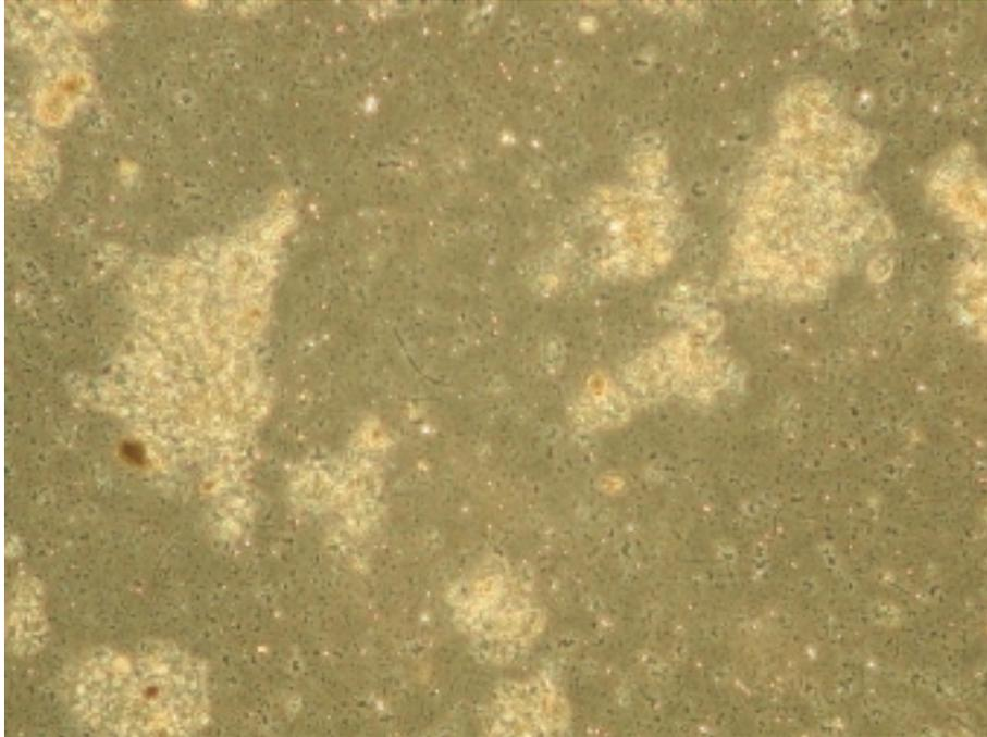
**Figure 5:** Light-microscopic image of sonicated sludge (specific energy input 0.2 kWh/kg<sub>TSS</sub>), enlargement factor 100, sample corresponds to figures 6a and 6b.
