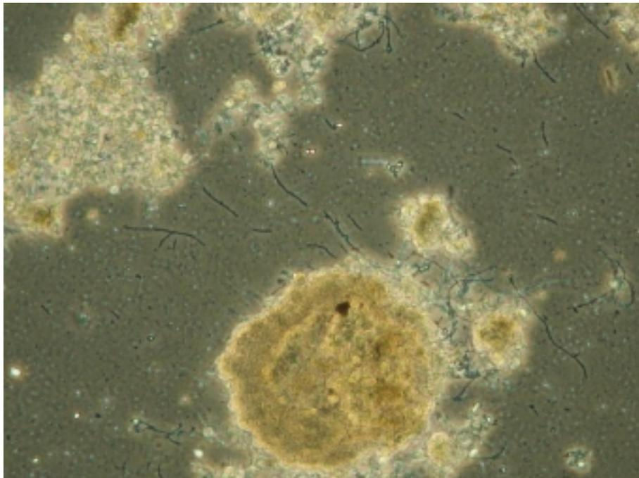
**Figure 4:** Light-microscopic image of sonicated sludge (specific energy input 0.05 kWh/kg<sub>TSS</sub>), enlargement factor 200, sample corresponds to figures 6a and 6b.
