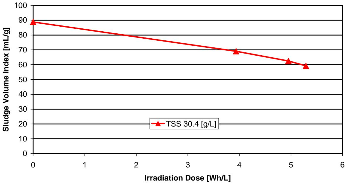
**Figure 9a:** Sludge volume index as a function of irradiation dose; samples from the STP Reinfeld, Germany. Full-scale.
