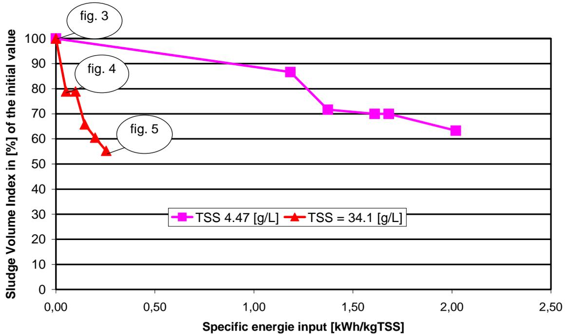
**Figure 7b:** Sludge volume index at different specific energy inputs; samples from the STP Reinfeld, Germany. Lab-scale.
